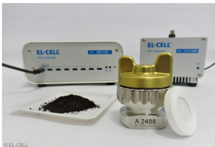
Fig. 1. PAT-Cell system, solid electrolyte and active material for sodium batteries in the KeNaB-ART project.
