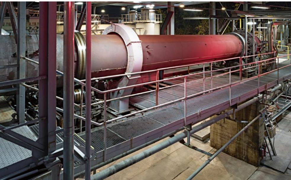
Figure 4 The directly fired rotary kiln (GDO) at IBU-tec (© IBU-tec)
