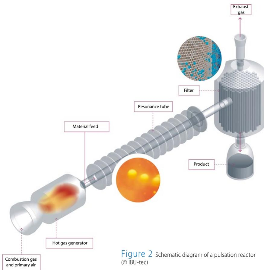
**Figure 2** Schematic diagram of a pulsation reactor
