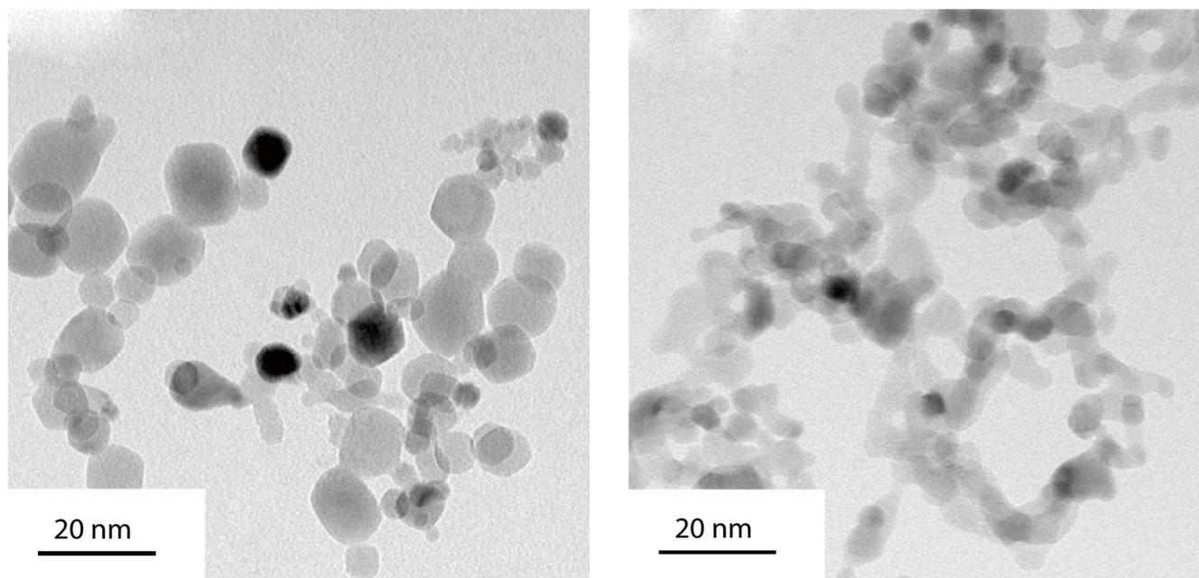
Figure 3 Transmission electron microscope images of  $ZrO_2$  from a flame spray pyrolysis unit (left) and a pulsation reactor (right) (© IBU-tec)
